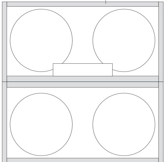
"Skinny" gold piping inside 1/8 x 1/8" dado, cut 1 11/16" from edge of cabinet (to the center of the dado) and extending across panel and into front and back edges. Does not extend inside cabinet.
