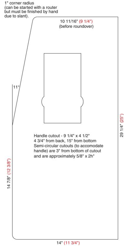
Note - baffle is cut 1/4" smaller (1/8" each edge) than the inside dimensions of the cabinet to accommodate grill.
